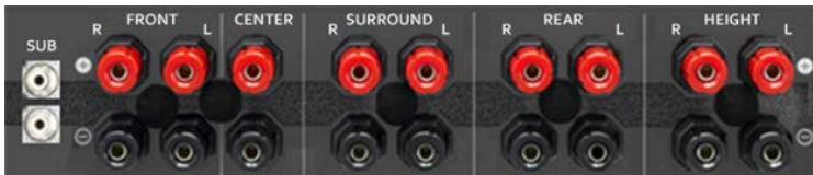
Figure 7: Rear panel of a 7.2.2 AVR; height speaker connections are at right.
